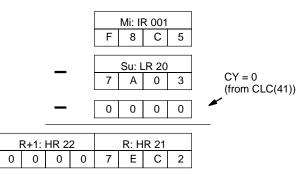
**Note** The status of the UF and OF flags can be ignored since they are relevant only in the subtraction of signed binary data.
